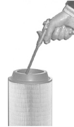
Fig4-4 Diagram for oil filter clean
